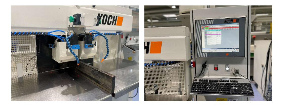
Stop and stock clamping system, workpiece detection and two-hand operation.
