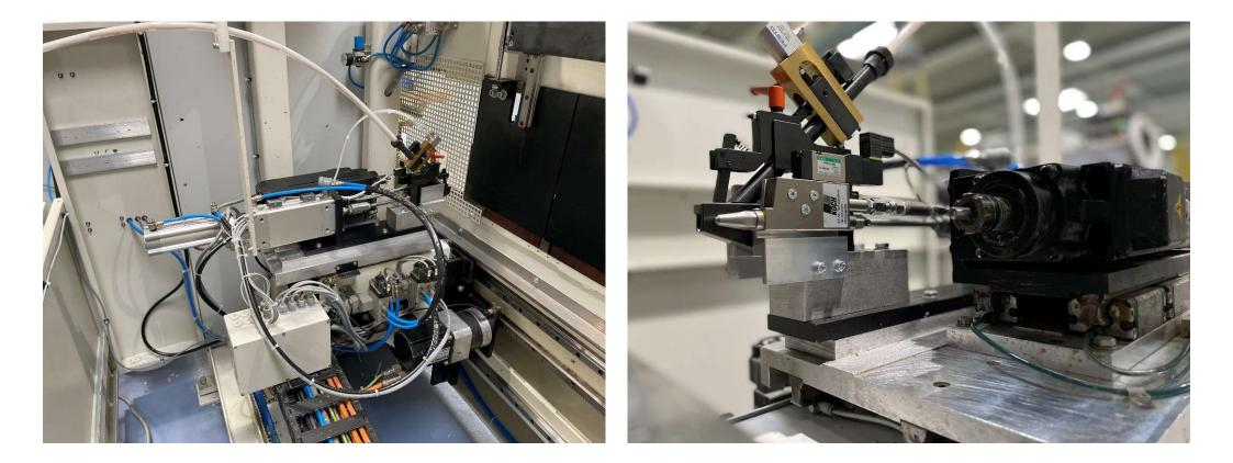
Support with horizontal drilling station, glue injecting and dowel insertion station Drilling motor, glue valve and dowel insertion tool
