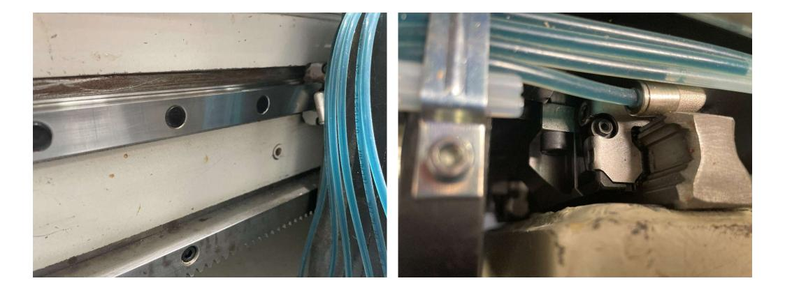
NEW linear guidance system on X and Z axes
