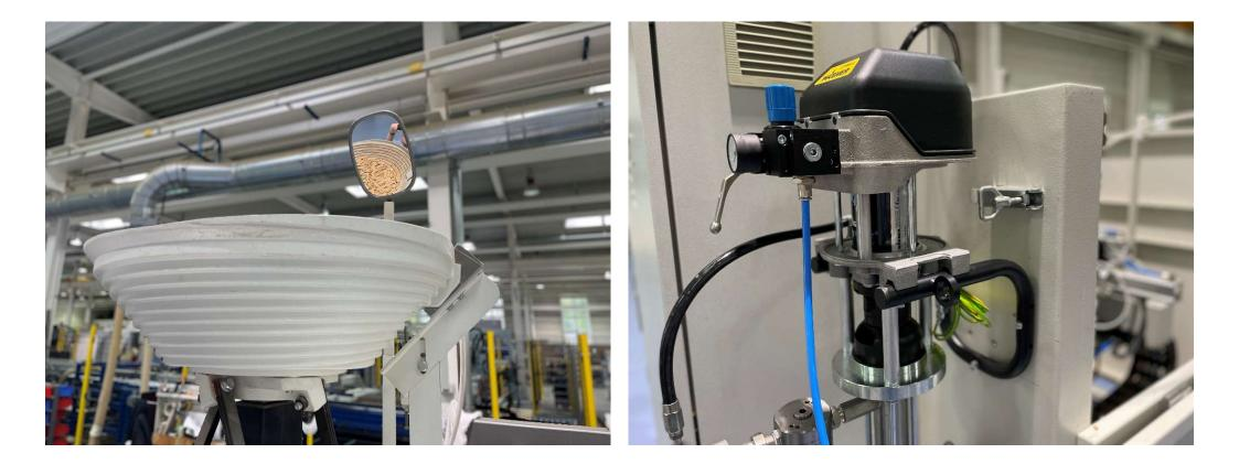
Control mirror for vibrator hopper conveyor
