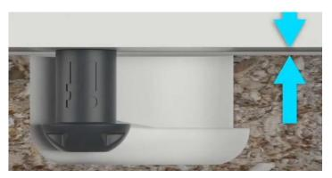
The PEANUT head has been specially designed to maximize ease of assembly and joint strength. Due to its dome shape, the PEANUT head smoothly slides along the slot created by the T-shaped PEANUT Cutter.
