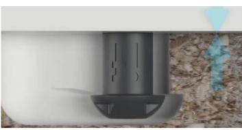
In assembly, the PEANUT head rides over the lip of the PEANUT slot and slides to the end, this action creates a strong clamping force, pulling the two panels together from the inside.
